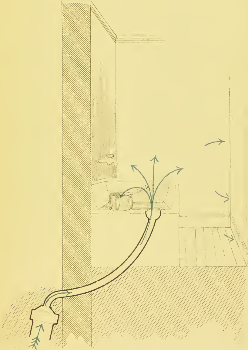
Waste pipe of kitchen sink untrapped, passing direct into drain.
